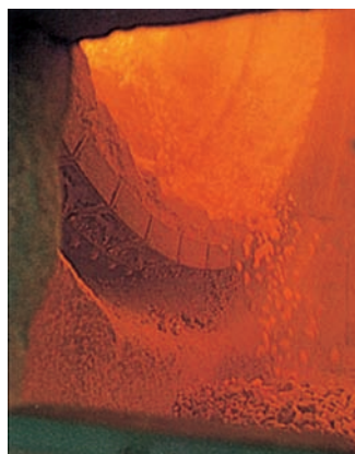
Figure 18.7 The production of CaO from \text{CaCO}_3 in a rotary kiln.
