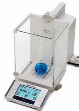
Figure 1.9 A single-pan balance.
