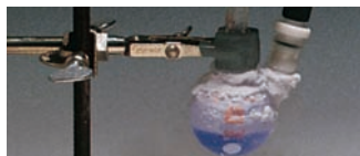
Liquid ozone below its boiling point ( -111.3^\circ\text{C} ). Ozone is a toxic, light-blue gas with a pungent odor.
