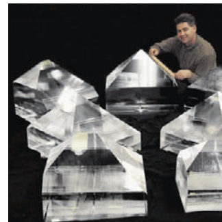
These giant ionic potassium dihydrogen phosphate crystals were grown in the laboratory. The largest one weighs 701 lb!
